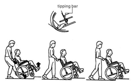
5. To move up or down a steep slope, ensure that a care giver is around to support the wheelchair; otherwise, the chair may overturn. For a steep downward slope, the wheelchair should be turned to face up slope, and the care giver should back the chair downwards gradually.
