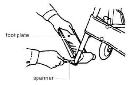
Using a spanner, slightly loosen the portion of the step pipe where it is bolted to the foot plate.
