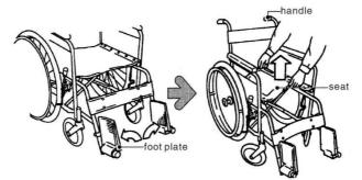
Flip the footplate upwards in the direction of the arrow. Lift the center of the seat up to fold the wheelchair.
